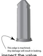
Then either the valve is damaged or the tee is not screwed into the trough firmly enough. Push the valve up and down a couple of times to see if you can dislodge anything that is stuck between the plunger seat and the valve body. If this doesn't remedy the problem, take the pipe out of the trough tee (push pipe in, turn a ¼ turn anticlockwise, pull). Undo the tee (noting the firmness of the fit) and visually
