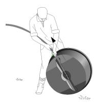
Push the Low Density Trough Lead firmly into the Trough Tee, making sure you push through the O-Ring but no so far as to disrupt the valve action. Because of the difficulty of doing this on an angle, we strongly suggest you mark the spot on the pipe (the pipe needs to go in the same distance as the cone). Once the trough lead is home, turn it clockwise and pull back firmly as indicated (you can also twist the trough anti-clockwise to achieve the turn)
