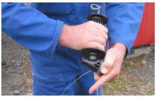
Step 4: Use hand and index finger as a brace when rotating Handle (also helps guide wrap).
