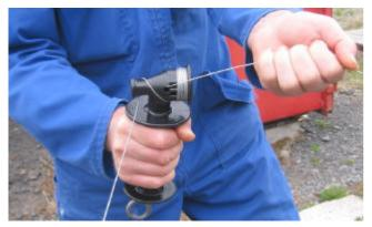
Step 7: Bend wire 'end' out of the way (towards the large drum of the Handle Strainer).
