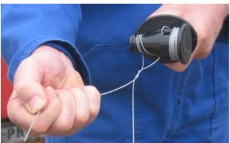
Step 10: Once tension has been decided, take the wire 'end' and 'lazy wrap' around the tensioned length. Finish off by kinking end.
