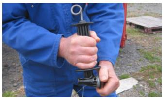
Step 5: Wind on enough wire to suit anticipated 'spare' requirements (the big drum was designed to be a wire reservoir to add length to the fence i.e. after fixing a number of breaks).
