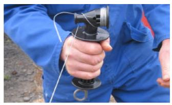
Step 6: When the large drum end of the Handle Strainer is 5cm from pulling up alongside the 'hook on point' of the Kiwitech or homemade thong take the wire over to the small drum.
