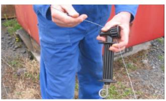
Step 2: Bend wire 'end' out of the way (towards small drum of Handle Strainer).
