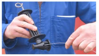
Step 1: Thread wire end (maximum diameter 2.5mm) through hole. Push through around 30cm.
